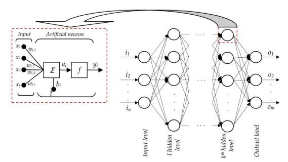
Figure 1 The structure of the feed-forward artificial Deep Neural Network (DNN) (image credit)
